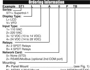
N= NEMA 4 Wall Mount .....(see NEMAtroIST4X) W= NEMA 12/13 Wall Mount w/ Clear Cover ...... (see Fig.2) E= Explosion Proof (No Button Access) ...... (see XHVD 7/4) X= Explosion Proof (with Button Access) ... (see XTROL 7/4) Options:
